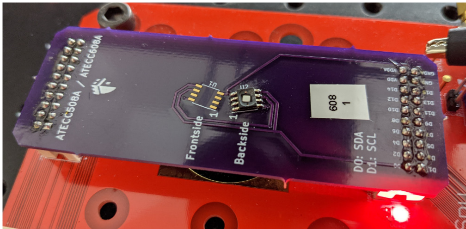
Fig. 2. Backside decapsulated ATECC608A chip, soldered on Scaffold daughter-board.
