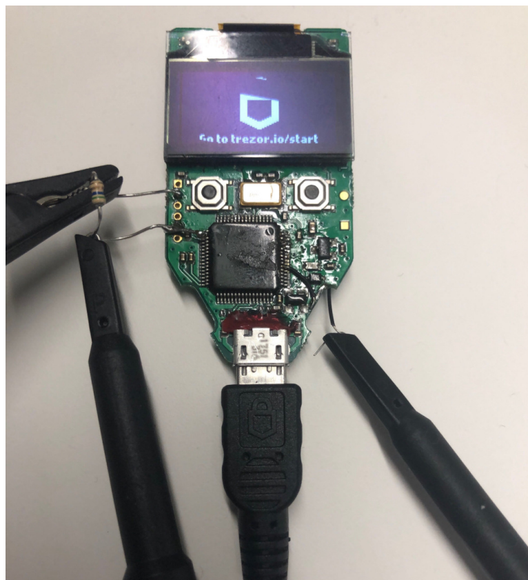
Fig. 3. Trezor One device prepared for side-channel: the probe to the left measures the power thanks to a resistor, and the probe to the right is plugged to a GPIO for triggering the scope.
